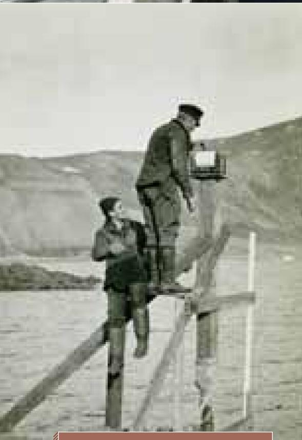
A Coast Survey officer checks an automated tide gauge. The white cylinder rotates constantly, recording the water's rise and fall minute by minute.
