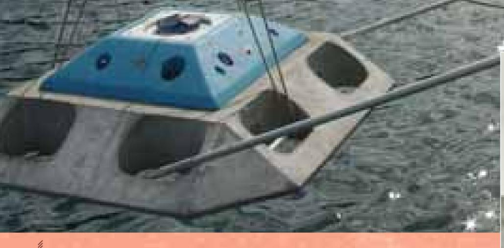
A Coast Survey crew lowers a continuouscurrent meter overboard near Sitka, Alaska. Equipped with an acoustic sensor, the meter measures the speed of particles carried in the current.
